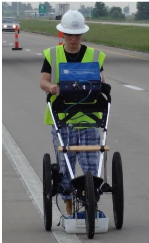
Figure 7-2 A MS&T Researcher Acquiring GPR Data with GSSI SIR-3000 GPR System with a GSSI 1.5 GHz Ground Coupled Antenna Along a Roadway Segment
