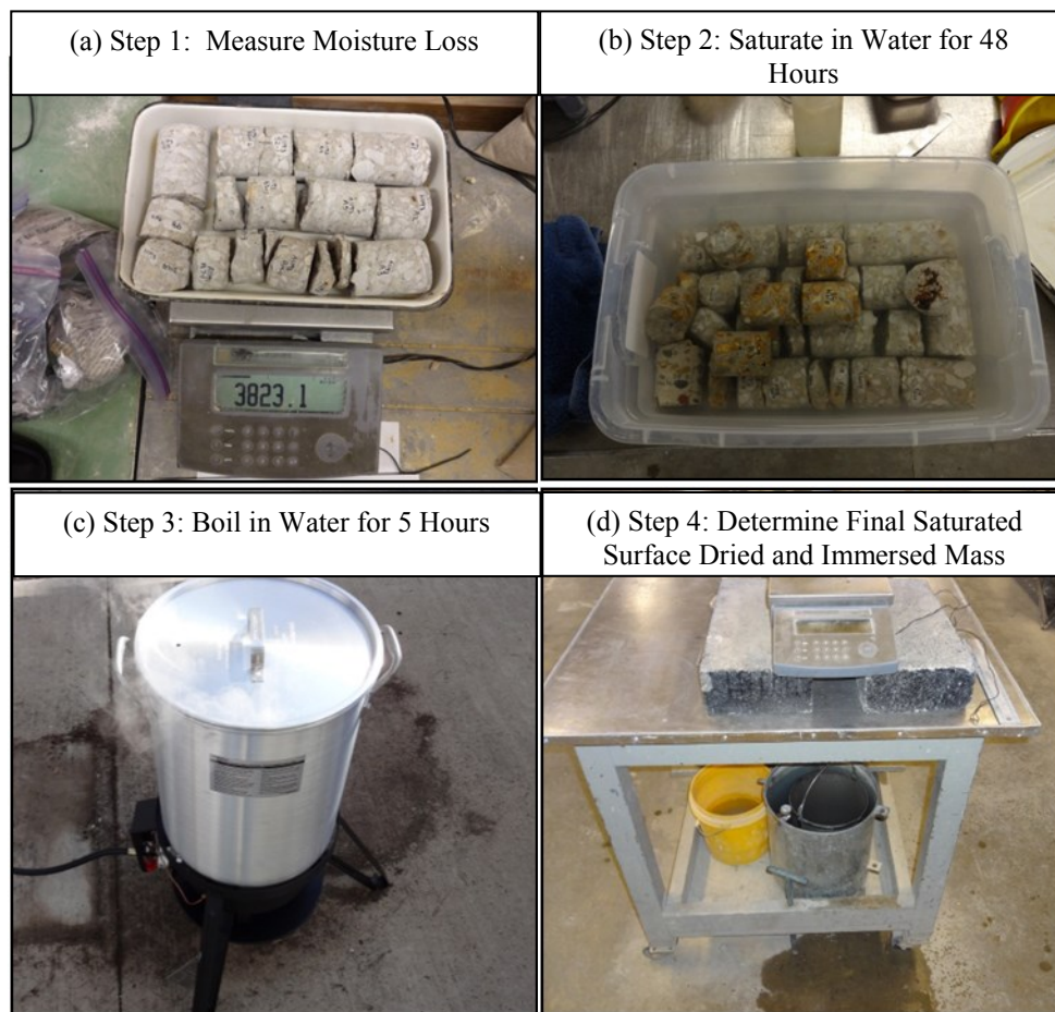
Figure 4-1 Process of Determining Volume of Permeable Pores
