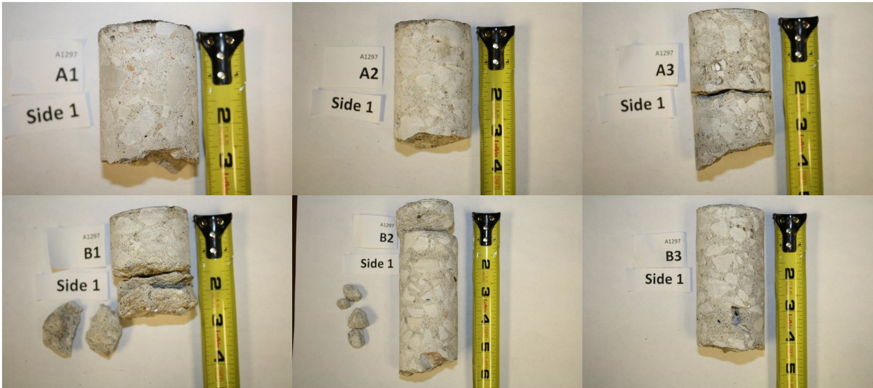
Figure 4-8 Cores Extracted From Bridge A1297
